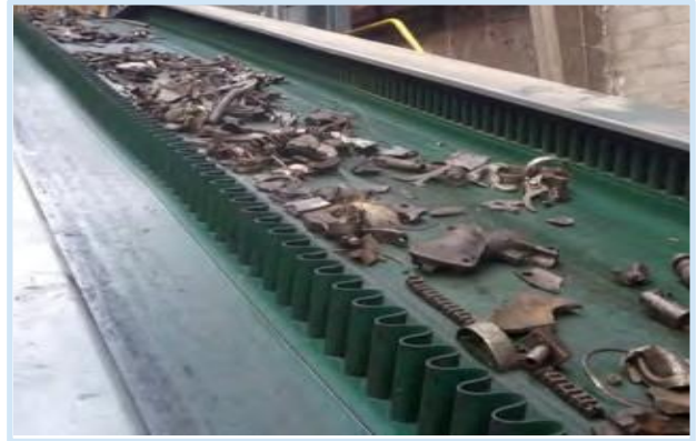
FRZ-5mm with welded Sidewalls: METAL RECYCLING
