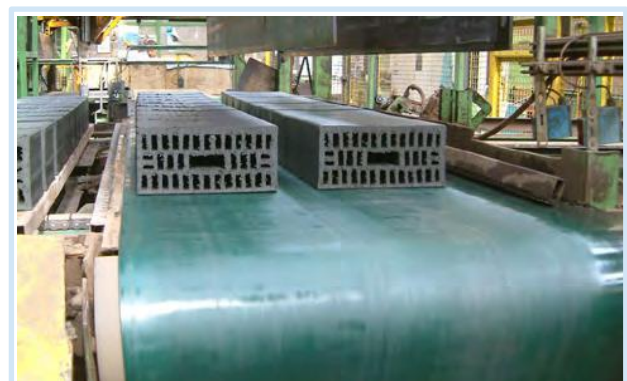
FRZ-4: HEAVY BRICK CONVEYING
