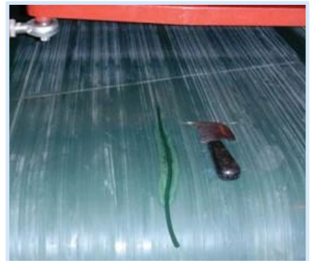
FRPZ-8 belt repaired with electrode
