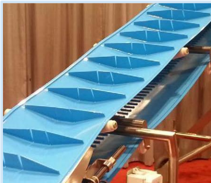
Special cleats on trough conveyor
