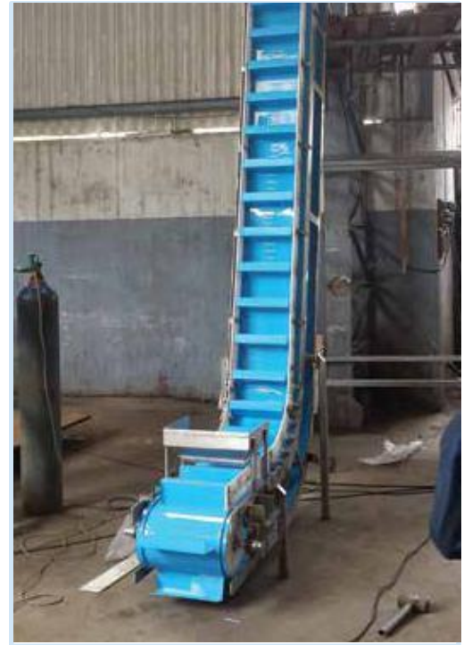
Fixed conveyor side wall
