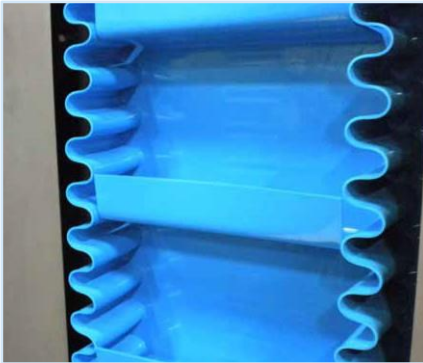
Integral welded side wall
