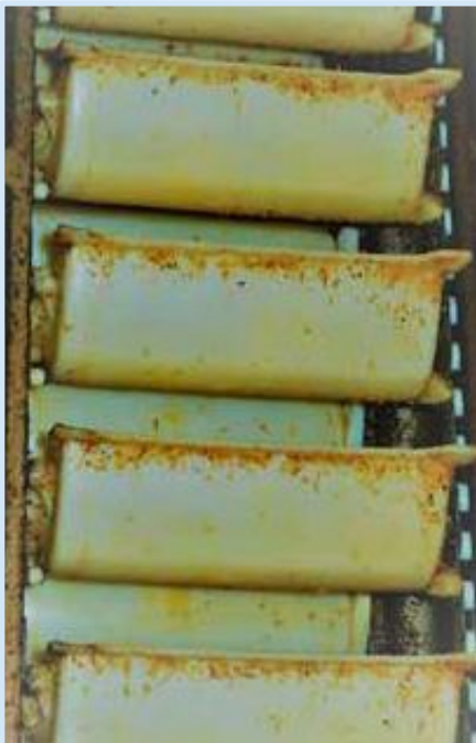
Open chain contaminated by food soil
