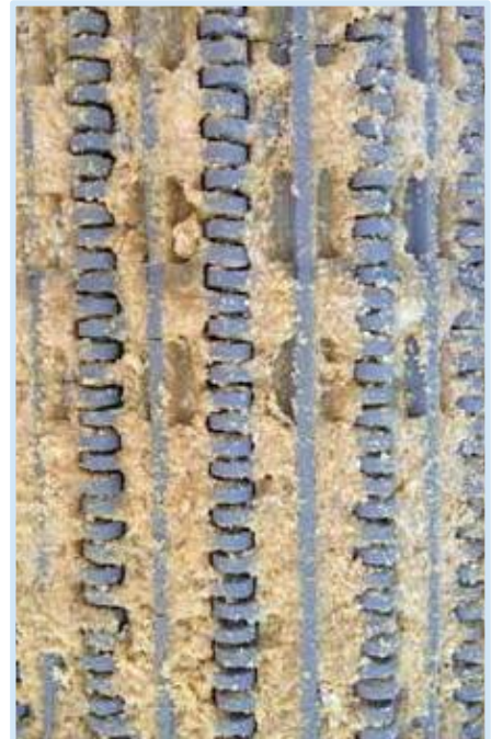
Bottom side of a modular belt
