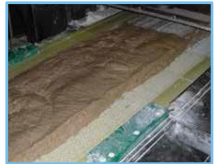
UHMW pieces holding 3mm Volta belt
