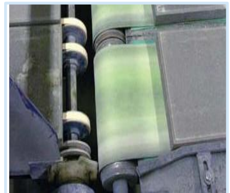
FK - 3 Brick pre - oven conveying
