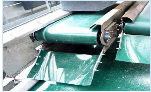
FRPZ-6 with Hammocks : PLASTIC PARTS CONVEYING
