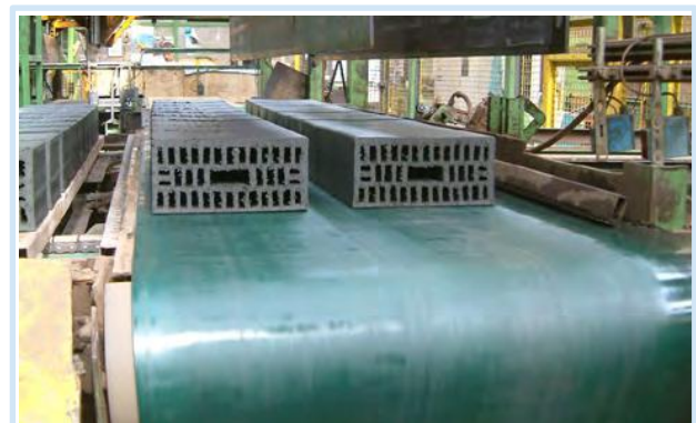
FRZ-4: HEAVY BRICK CONVEYING
