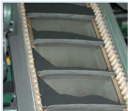
FRG - 3 Chemical powder conveying
