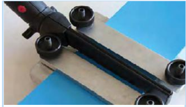
Welding narrow flat belts with Pliers P-200
