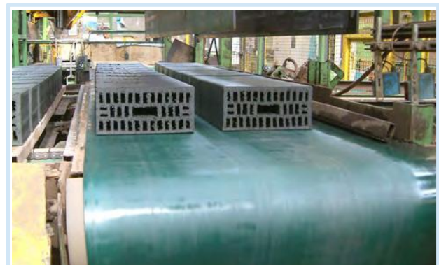
FRZ-4: HEAVY BRICK CONVEYING
