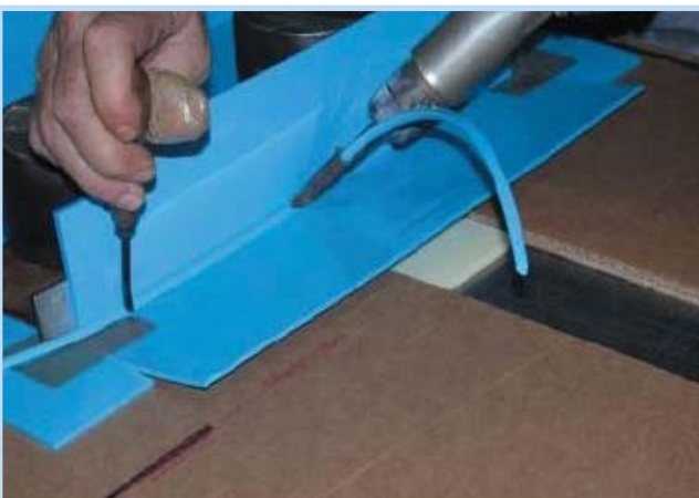
Electrode welding of cleats
