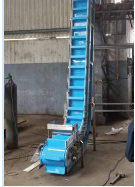
Fixed conveyor side wall
