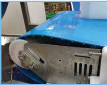
UHMW roundel mounted on pulley
