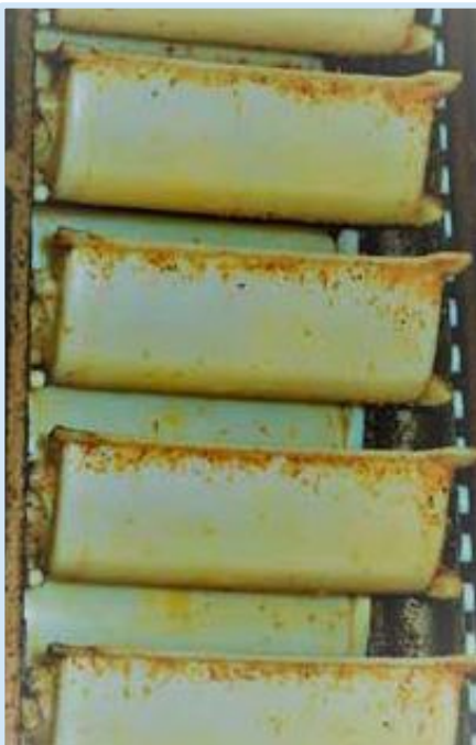
Open chain contaminated by food soil
