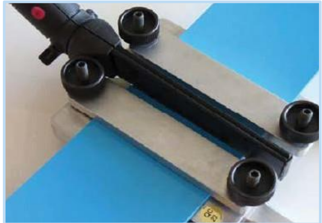
Welding narrow flat belts with Pliers P-200
