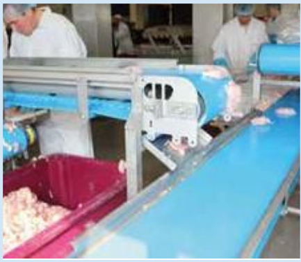
SuperDrive™ on portioning line
